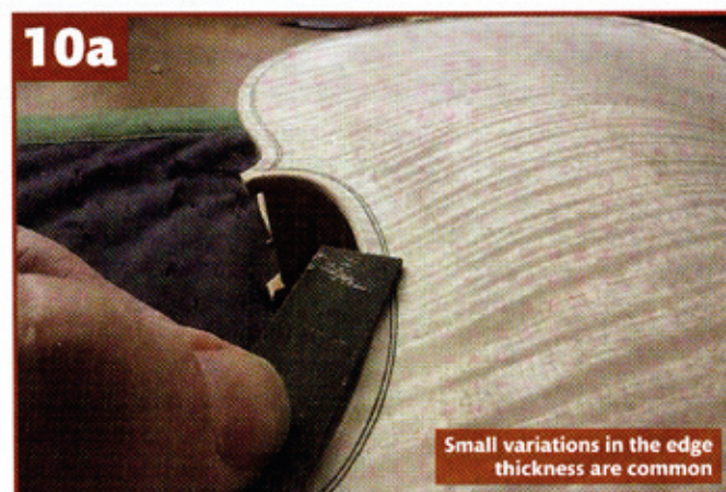
Sanding the edge with carefully folded sandpaper
